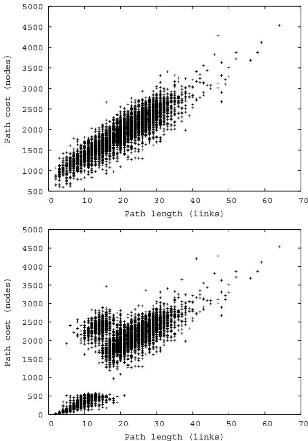
**Figure 2.** Comparison of the HTAP algorithm to the hybrid algorithm. Above, the hybrid algorithm; below, the hybrid algorithm. For short paths, the hybrid is superior, while for long paths, the two algorithms are identical. There may be a set of intermediate paths where the hybrid algorithm requires more work.
