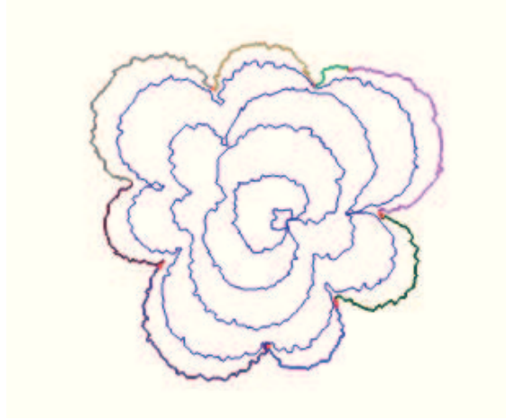
Figure 3.11 A result of linear interpolation over each curve. The linear interpolation is computed over the curve by setting the middle of the curve as the maximum input velocity and the corners at zero. Note that the inner contours are for illustrating and visualizing the growth process and that different curves are visualized with different colors for simplification.
