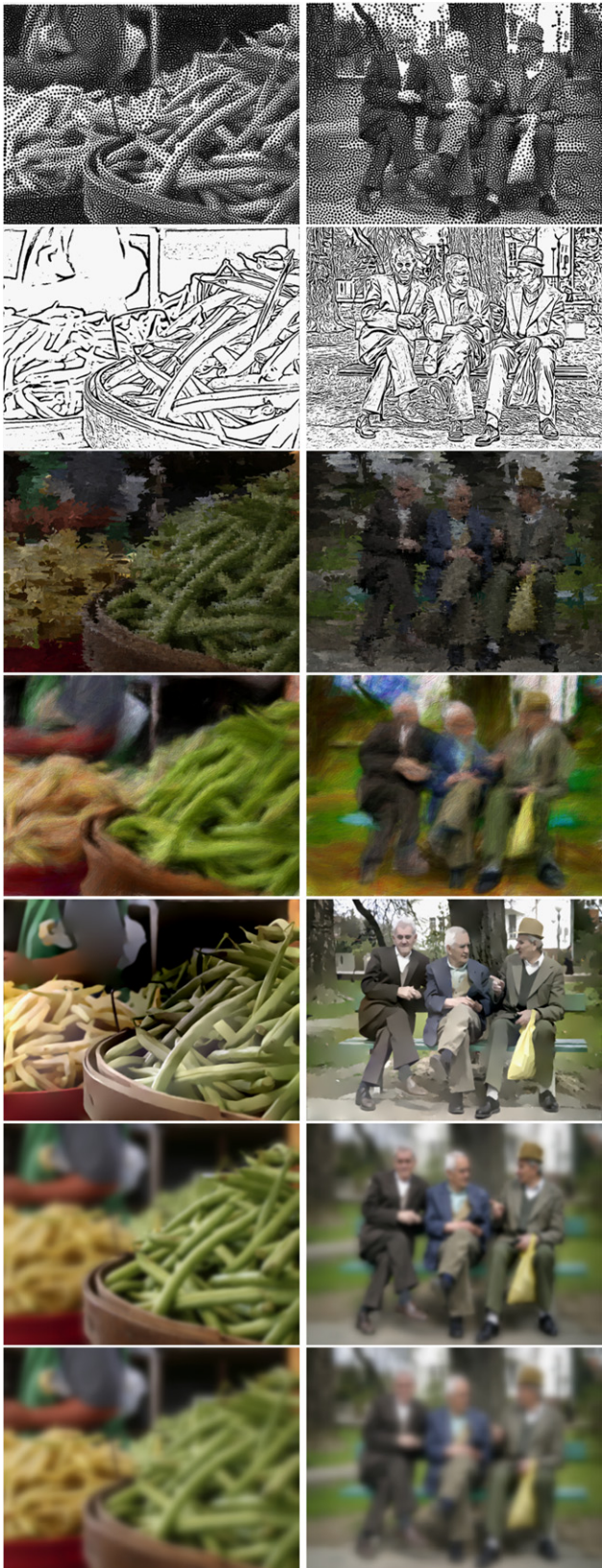
Fig. 4. Output from the rendering algorithms. From the top: stippling (Secord); line drawing (Kang); painting (Haeberli); painting (Sisley); photo abstraction (Orzan); object blur; uniform blur.
