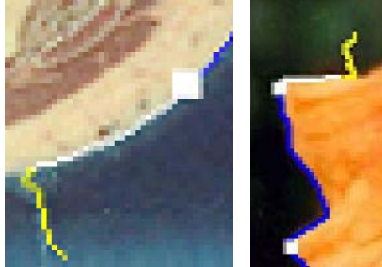
Figure 2. Two details illustrating the leash. Pixels known to be on the edge are colored blue. White indicates pixels probably on the edge and yellow indicates pixels the software is unsure about. Notice some yellow pixels are on the edge.
